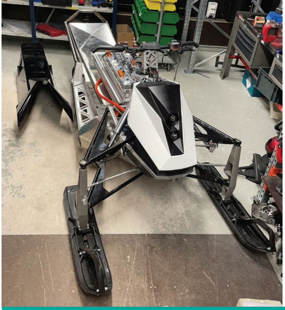
The new eSled, pictured here in Aurora’s workshop, has been designed in-house from a blank sheet for far superior range, battery capacity, comfort and handling than the first model
